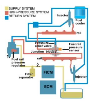
1. High-pressure pump is driven by the camshaft, but no timing marks are necessary.
